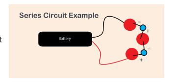
• **Answer**: This is a **series circuit** in which the LED closest to the power source has best access to the power source. The more LEDs there are, the less "push" each one gets. When there are too many, they no longer turn on. Usually more than 2 or 3 will not light up in a series.
